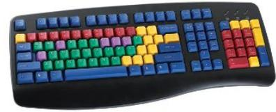
Alternative keyboards can support typing with features such as large keys, keyguards or coloured keys.
