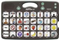
The Go Talk Express is a new static display communication device. It has 32 cells and 5 recording levels. This device can operate in a standard mode like other Go Talk devices, or in a sequenced mode where the user can combine words and say them all together in a more fluent manner when building sentences. This device also has one and two switch scanning capabilities, with visual and auditory feedback.
